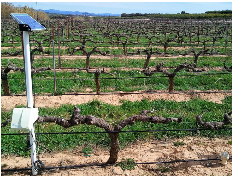
Picture 4: A soil moisture sensor capacitance probe installed in an irrigated vineyard (Credit D. Intrigliolo)
